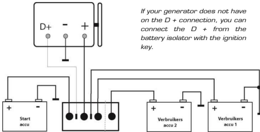
If your generator does not have on the D + connection, you can connect the D + from the battery isolator with the ignition key.
